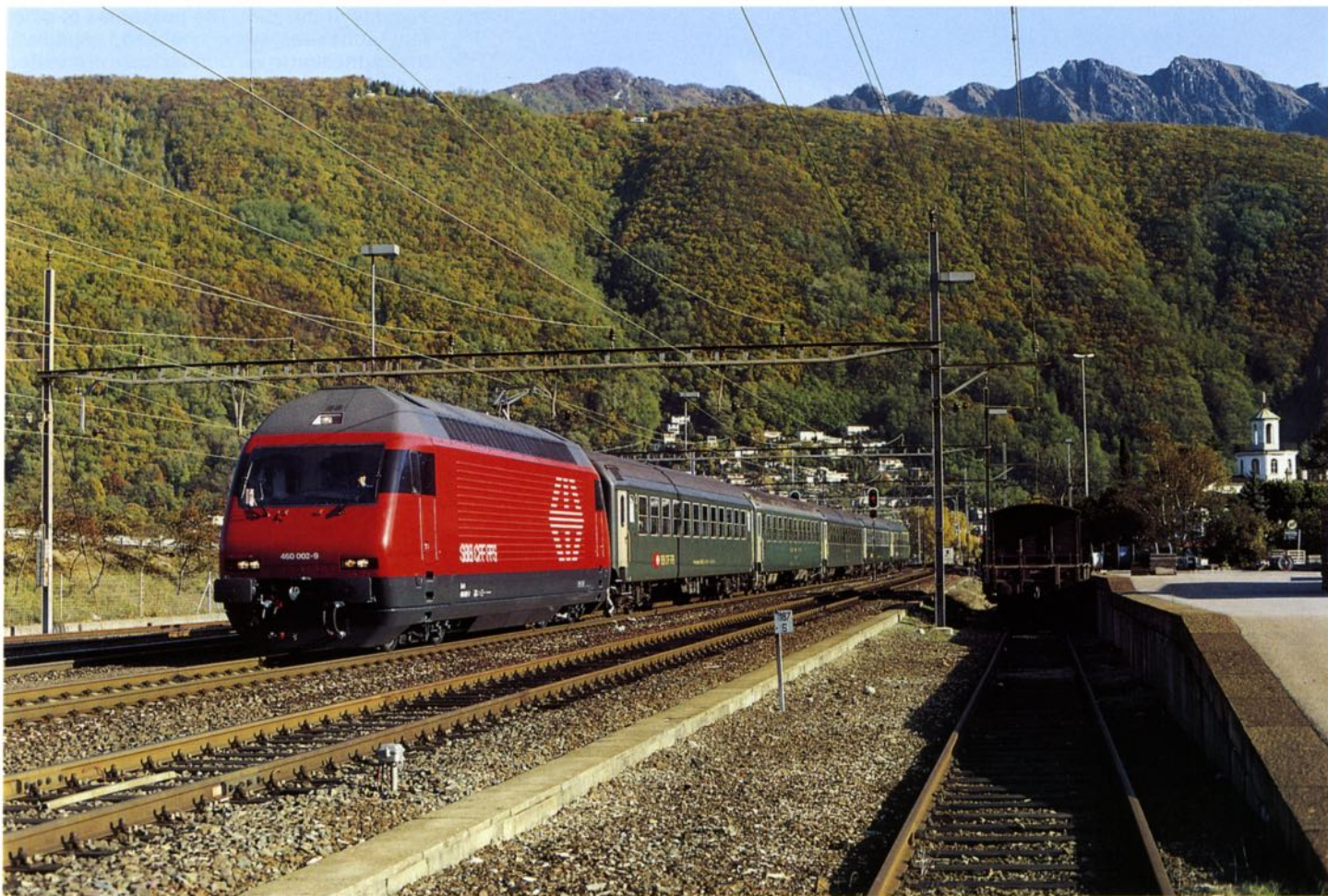
The finished locomotive 2000 on the track to the Gotthard near Melide. The external view gives no clue that it is made partly of plastic and partly of steel (Photo F. Suter 10.11.1991).
